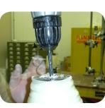
Rough up the surface of the PETG. Clean with rubbing alcohol (do NOT use acetone). Do a thin lamination over the PETG.
