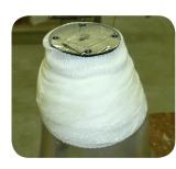
Drill a 9/32" hole in the socket.
