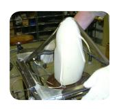
Tape off the hole in the 4-Hole Adapter. Tape off any holes in the socket.
